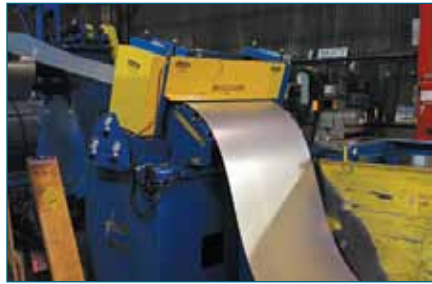
The steel is leveled through a straightener.
