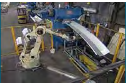
The finished panel is transferred by a robotic arm onto a pallet ready for shipment.
