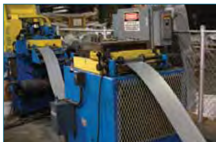
The steel is leveled through a straightener and punched by a state-of-the-art punching system.
