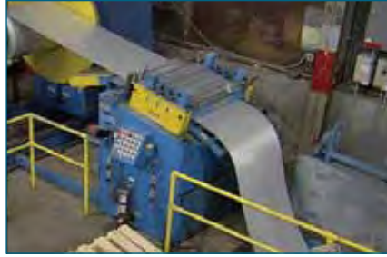
The steel is leveled through a straightener.
