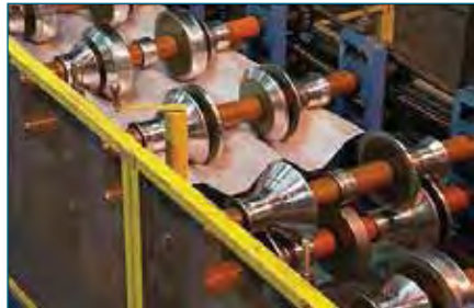
The cut sheets are shaped through a roll-forming process.
