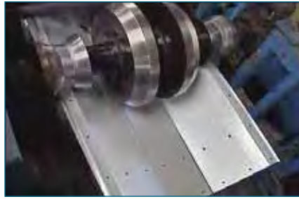
The cut sheets are shaped through a roll-forming process.
