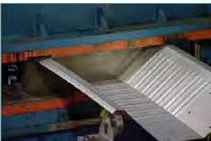
The panel is fed from the conveyor into the crimping machine where a radius is applied.
